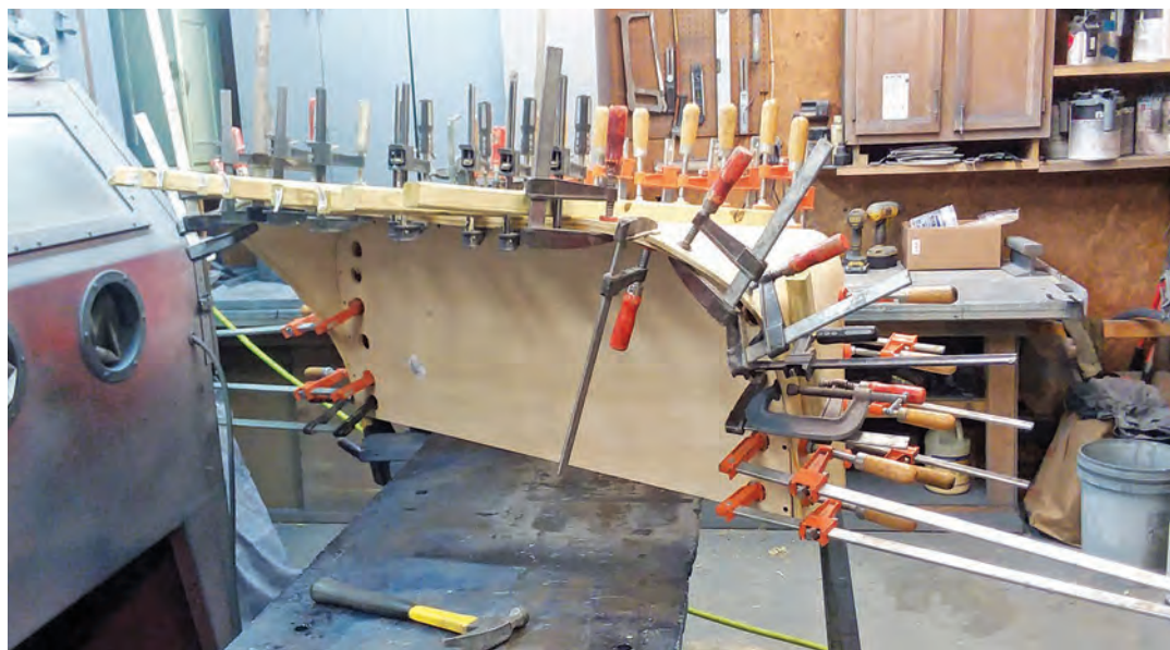
Photo 4: The glued up plywood sandwich clamped around seat bottom pattern.
