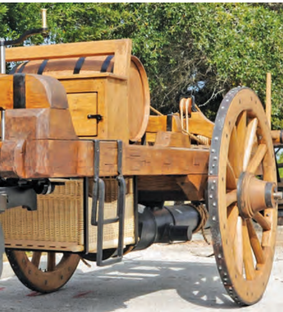
The wood-spoked wheel on the 1771 Cugnot reproduction illustrates an early vehicle wheel. (Photo courtesy of the Tampa Bay Auto Museum)
