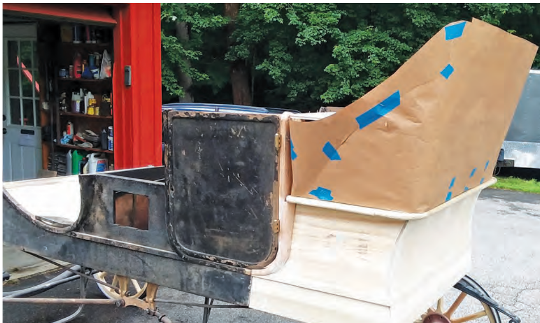
Photo 2: The paper pattern wrapped around the seat pattern.
