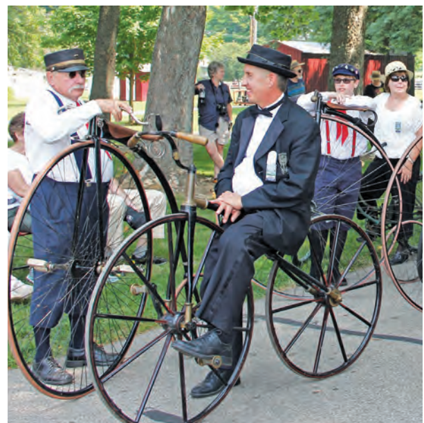
Two early pedal bikes; the wooden Velocipede circa 1870 with wood wheels and the ordinary bike circa 1888 with solid rubber tires and 60" wire wheels. (Image courtesy of David O. Lyon)
