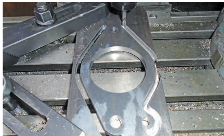
Figure 10. Cutting out the piece that is used to stiffen the flange of the starter motor.
