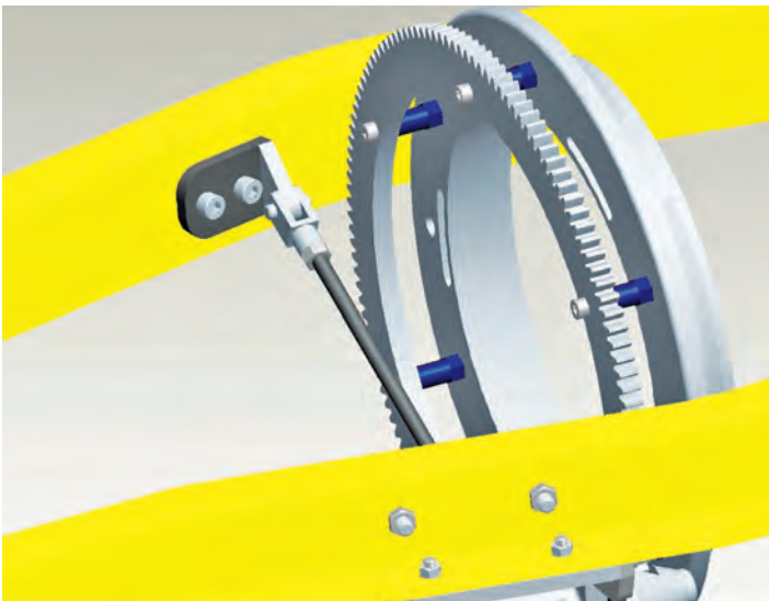
Figure 7. CAD view showing tie rod anchor and how the main bracket is fixed to the chassis.
