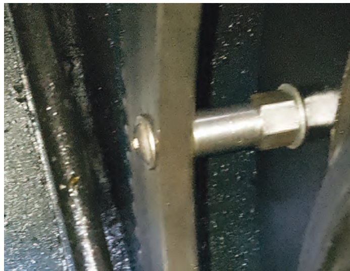
Figure 4. The ring gear is mounted on six spacers.
