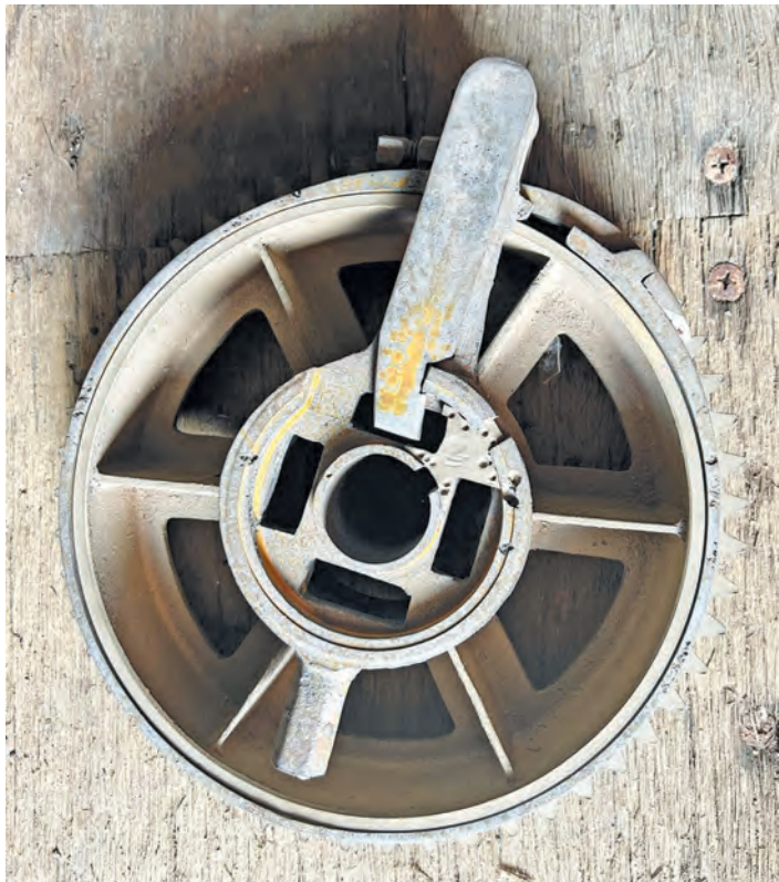
Above: This is our surrey's reverse gear. Note the four rectangle holes in the centre which house the gear engaging fingers and the arm that partially covers one hole, connected to the band on the outside of the gear, as the finger passes the arm it forces the band to contract (planetary transmission but internally operated), grabbing the gear, and locking it in mesh with the crankshaft. Below: The surrey's beautifully restored tiller.
