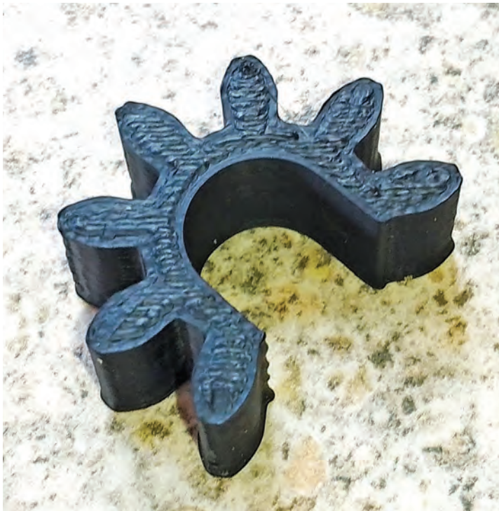
Figure 11. "Clip on" pinion gear printed in plastic.
